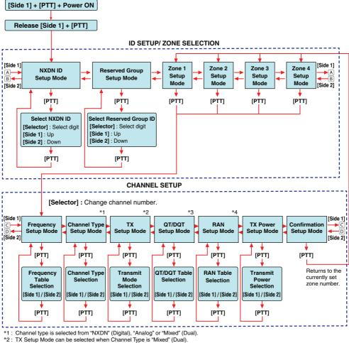
\*3 : QT/DQT Setup Mode can be selected when Channel Type is "Analog" or "Mixed" (Dual).
